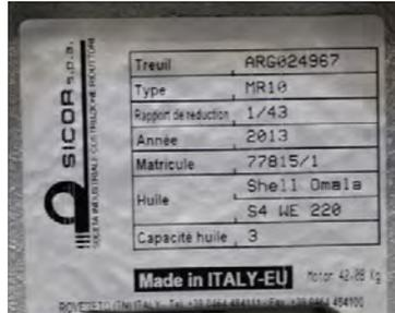
You can also find on this label essential information such as the type of machine, the reduction and the type of oil.
